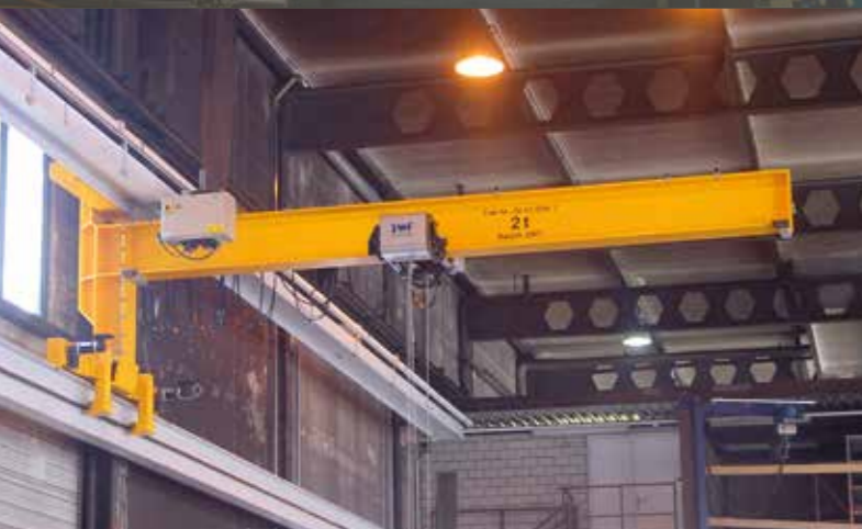
Wall console crane
