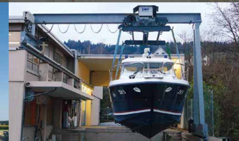
Semi gantry crane
